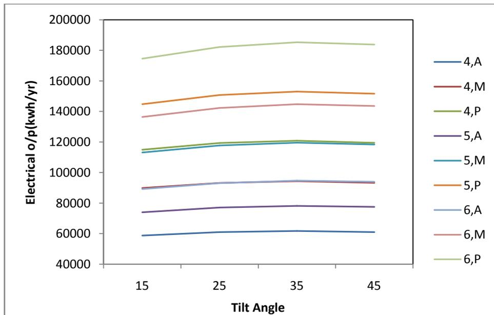
Figure 4: Effect of tilt angle, type of cell and radiation level on electrical output(kWh/year) for  $\phi=34^\circ$ .
