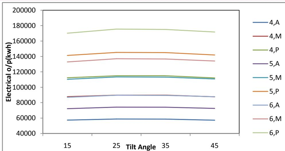
Figure 5: Effect of tilt angle, type of cell and radiation level on electrical output (kWh/year) for  $\phi=26^{\circ}$ .
