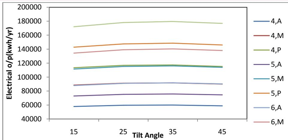
**Figure 1.** Effect of tilt angle, type of cell and radiation level on electrical output (kWh/year) for location with  $\phi=28^\circ$ .
