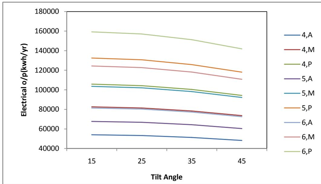
Figure 3: Effect of tilt angle, type of cell and radiation level on electrical output(kWh/year) for  $\phi=12^\circ$ .
