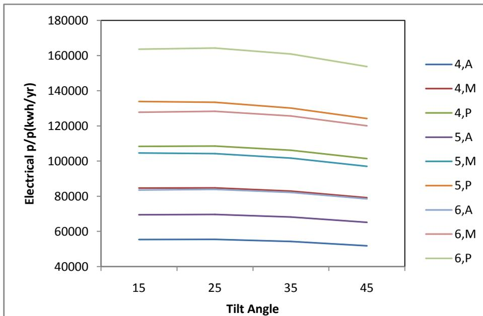
**Figure 2:** Effect of tilt angle, type of cell and radiation level on electrical output(kWh/year) for  $\phi=18^\circ$ .
