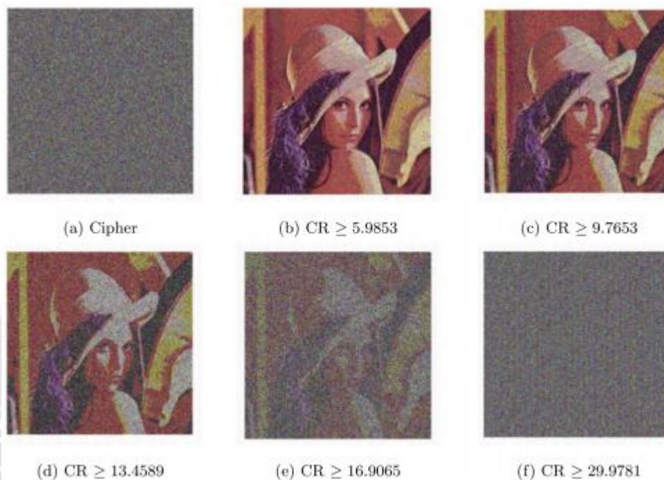
Fig. 10. Compression Ratio (CR) test (Lossless). (a) Cipher image, (b) CR \geq 5.9853 , (c) CR \geq 9.7653 , (d) CR \geq 13.4589 , (e) CR \geq 16.9065 , (f) CR \geq 29.9781 .
