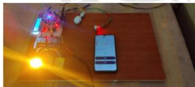
Fig.8. When temperature is controlled the LED no.1 glows as output.
