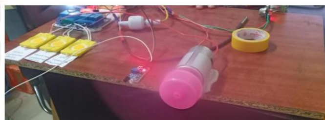
Fig.10 Controlling of the Motor /Fan
