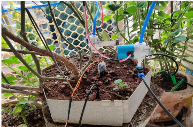
Figure 11. Fig. 10. The setup of our plant with the valves and sensors
