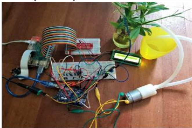
Figure 1. Raspberry Pi and Arduino to show the sensor values on an LCD Display monitor [14].
