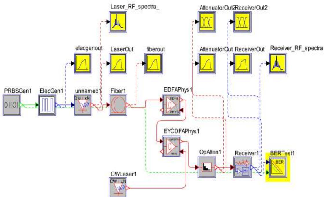
**Figure 4: Simulation Setup using Cascaded EDFA-EYCDFA**
