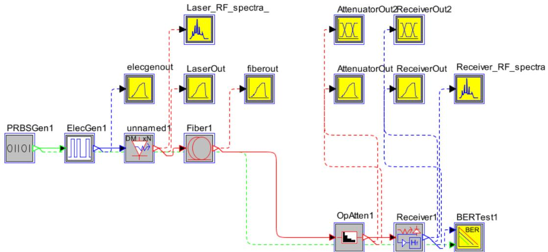
**Figure 3: Simulation Setup of 60 Gbps Single Channel Optical Link**
