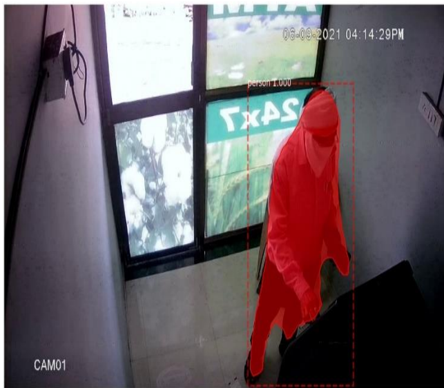
Figure 6. Output of Mask-RCNN object detection module
