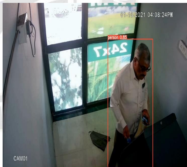
Figure 5. Output of YOLOv4 object detection module
