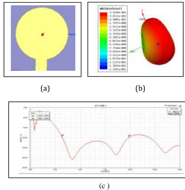
**Fig3:** (a)patch antenna design (b) gain in db (c) return loss graph
