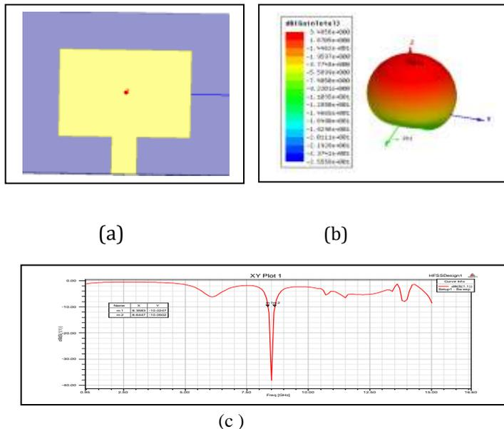
**Fig -1:** (a) patch antenna design (b)gain in db (c) return loss graph
