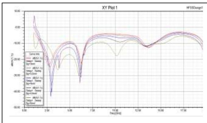
**Fig 2:** parametric Analysis of Ground Plane
