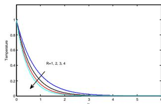
Fig.8.Temperature profiles for different values of radiation parameter (R).
