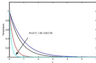
Fig.6.Temperature profiles for different values of Prandtl number (Pr).
