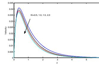
Fig.11.Velocity profiles for different values of chemical reaction parameter (Kr).
