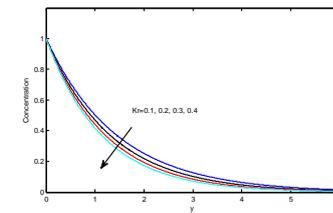
Fig.12.Concentration profiles for different values of chemical reaction parameter (Kr).
