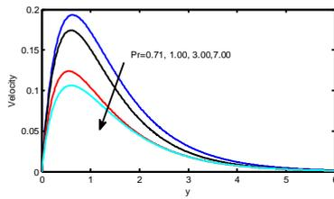
Fig.5.Velocity profiles for different values of Prandtl number (Pr).
