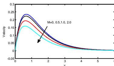
Fig.1.Velocity profiles for different values of magnetic parameter (M)
