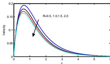
Fig.7.Velocity profiles for different values of radiation parameter (R).
