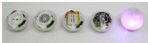
Fig 10 Interior structure of Phixel
