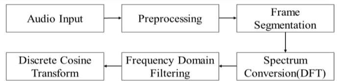
Figure 8. Flowchart representing different processes for extracting MFCC features from audio data.
