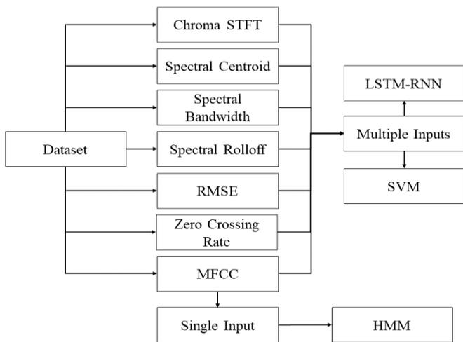
Figure 1. Flowchart representing a step by step procedural flow of the proposed system.
