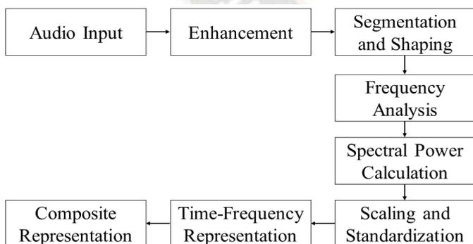
Figure 9. Flowchart representing different processes for extracting spectrogram features from audio
