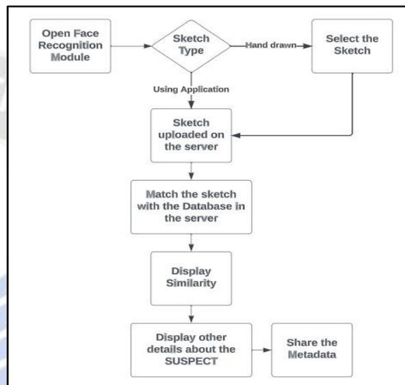
Fig. 2. Flow Diagram for Sketch Recognition
