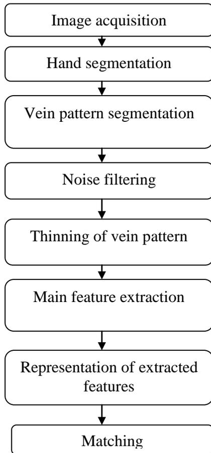
**Fig.4 Biometric Procedure**
