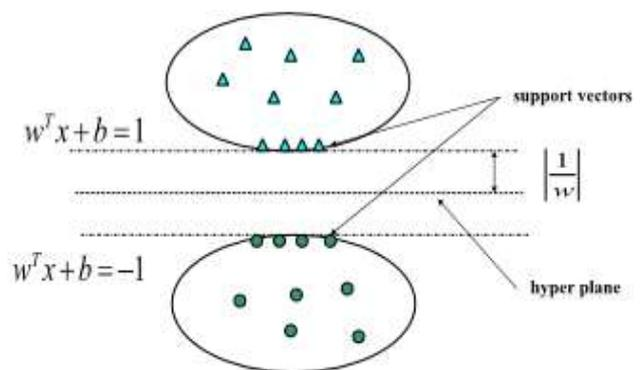
**Fig.5 A linear separable Support Vector Machine**
