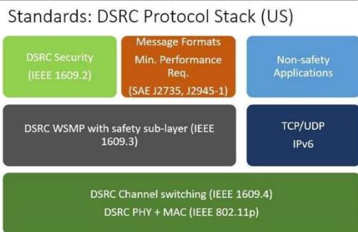
Figure 1. DSRC Protocol Stack
