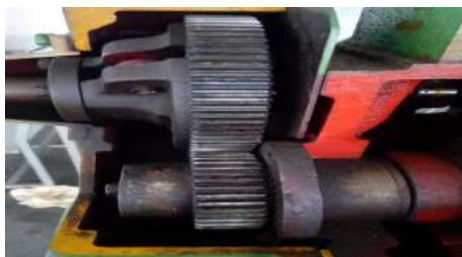
Figure. 2. Improper Chamfering
