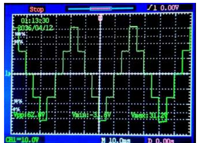
Figure 4.6: Output Voltage Waveforms on DSO with Vpp , Vmin and Vmax
