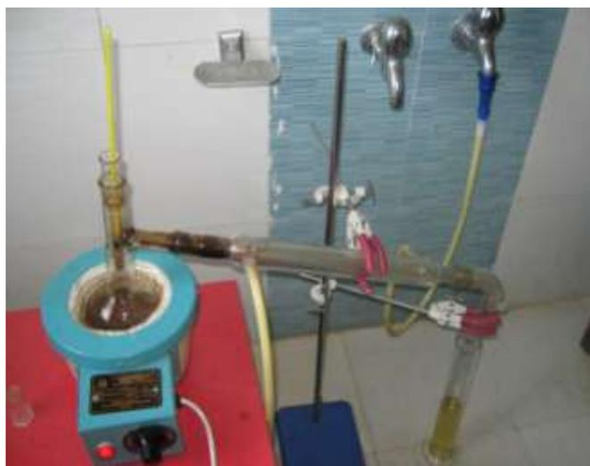
Fig. 2 Distillation Apparatus
