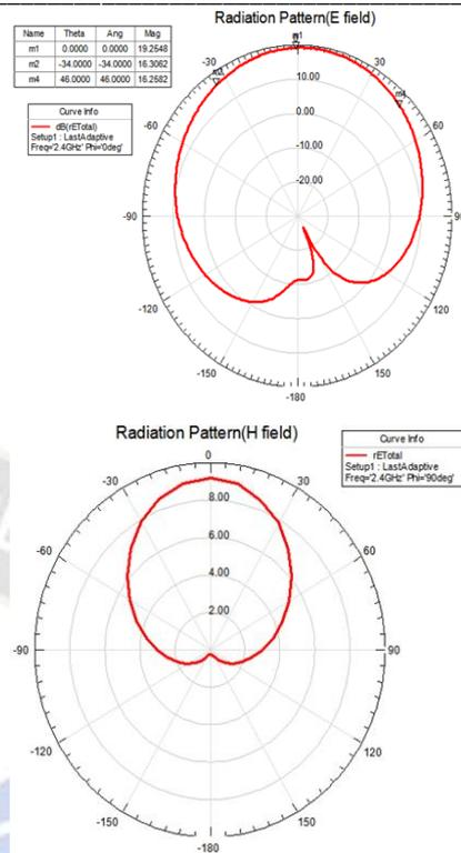
Fig. 4. 2D Radiation pattern; (a) E field radiation pattern, (b) H field radiation pattern
