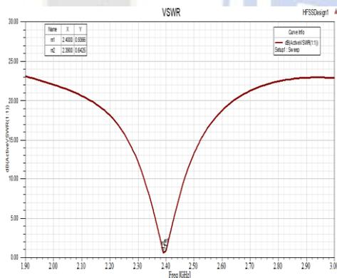
Fig. 3. VSWR versus frequency plot of the patch antenna
