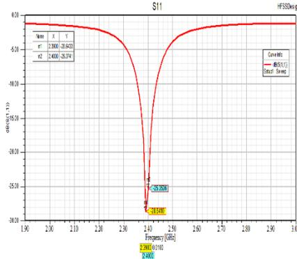
Fig. 2. Return loss versus frequency plot of the patch antenna.
