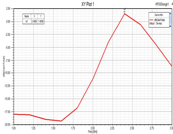
Fig. 6. Gain versus frequency plot of the patch antenna
