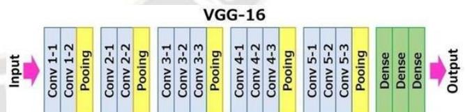
Figure 5. Architecture of VGG-16 model
