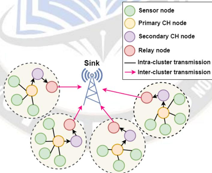
Figure 2. WSN Architecture using WMCL-DLRS-CRP
