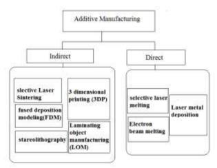
Fig 1: Different Additive Manufacturing Technologies
