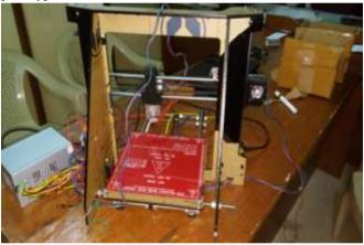
Figure 5 Experimental setup of Wireless 3D Printer prototype
