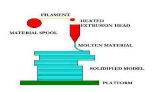
Fig 3: Molten material coming out of nozzle and deposited layer by layer.
