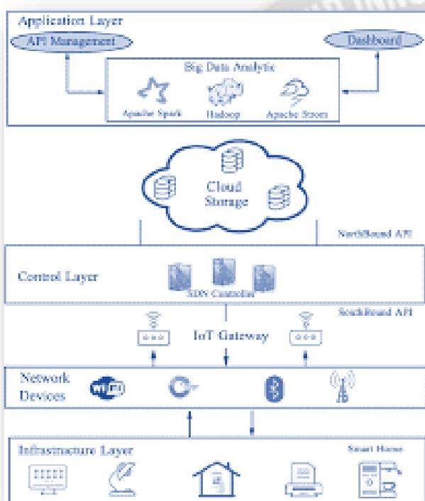
Figure 1: Architecture of IoT-SDNCT
