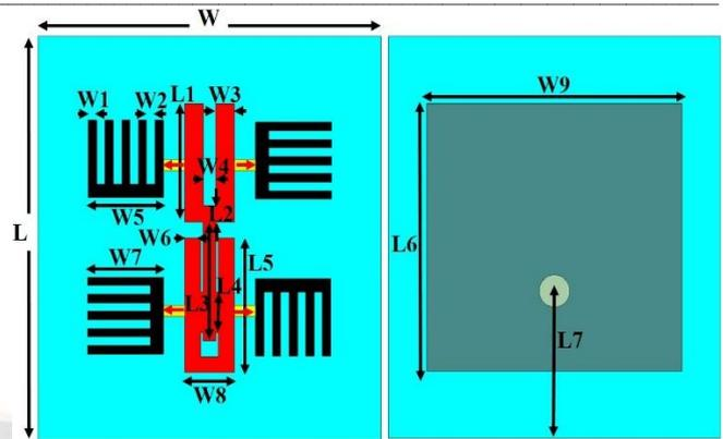
Figure 1. Pattern reconfigurable antenna model: (a) Top view; (b) Back view.
