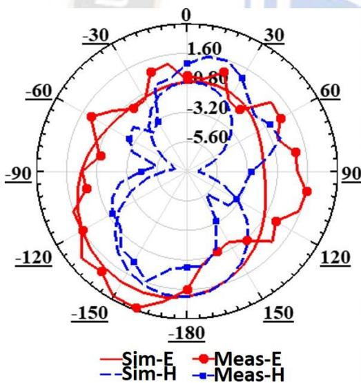
Figure 13. Comparison of E and H plane radiation patterns between simulations and measurements
