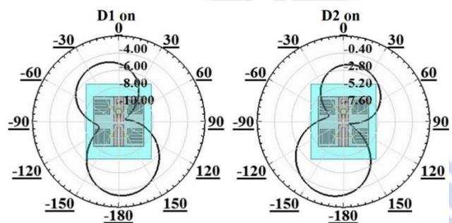
Figure: 7 Radiation pattern comparisons a) Only D1 ON & b) Only D2 ON
