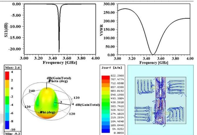
Figure: 4 Antenna simulated performance when all diodes are off a) Reflection coefficient b) VSWR c) 3D radiation plot & d) Current field distribution
