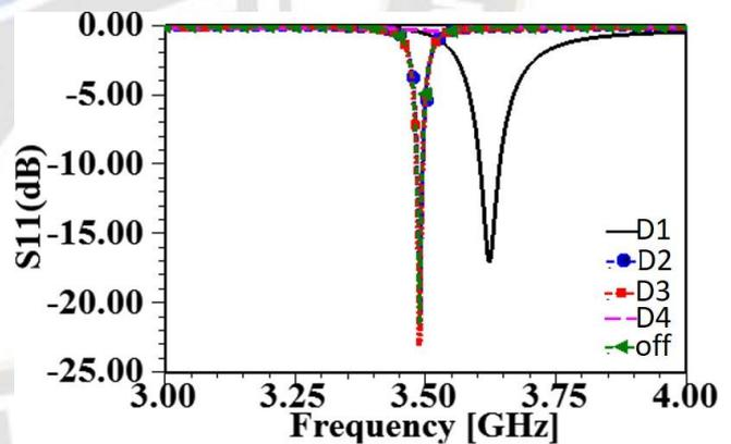
Figure: 5 Reflection coefficient comparison when each of the diodes is on with all diodes off condition
