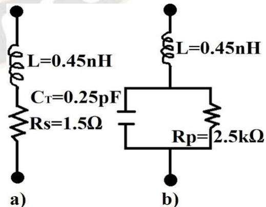
Figure: 2 Forward and reverse Bias Conditions for BAR-64-02V
