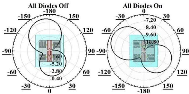
Figure: 6 Radiation pattern comparison a) All diode OFF & b) All diodes ON
