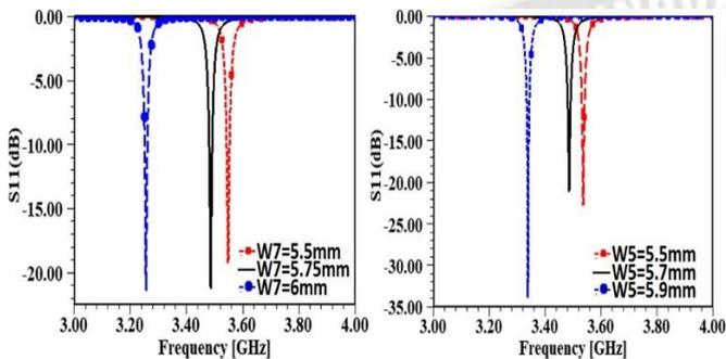
Figure: 3 Reflection coefficient comparison a) Parametric study for W7 & b) Parametric study for W5
