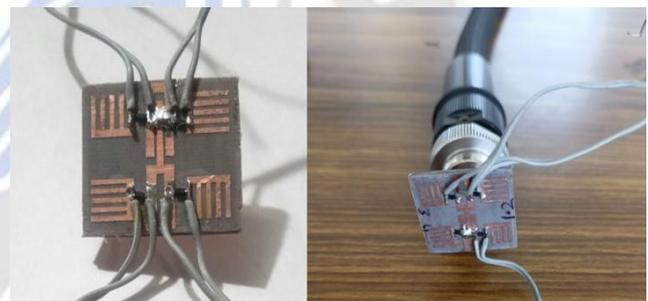
Figure: 10 Pattern reconfigurable antenna for 5G n78 band: Fabricated prototype
