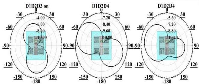
Figure: 9 Radiation pattern comparison a) D1D2D3 ON & b) D1D2D4 ON & c) D1D2D4 ON
