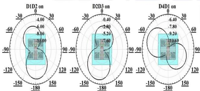
Figure: 8 Radiation pattern comparison a) D1 & D2 ON & b) D2 & D3 ON & c) D4 & D1 ON
