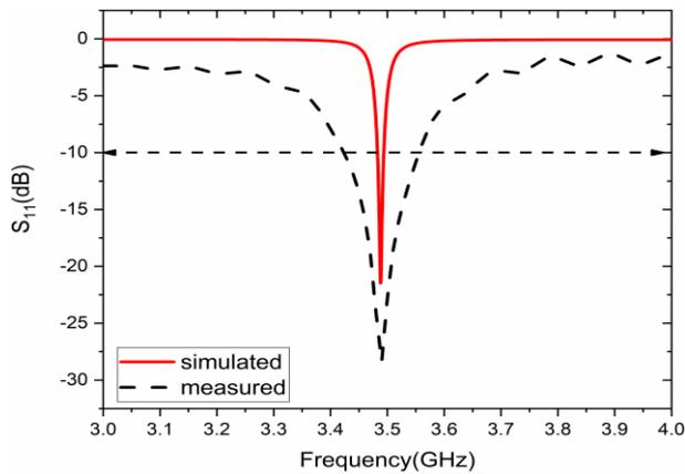
Figure 12. Reflection coefficient: Comparative study that is simulated and measured
