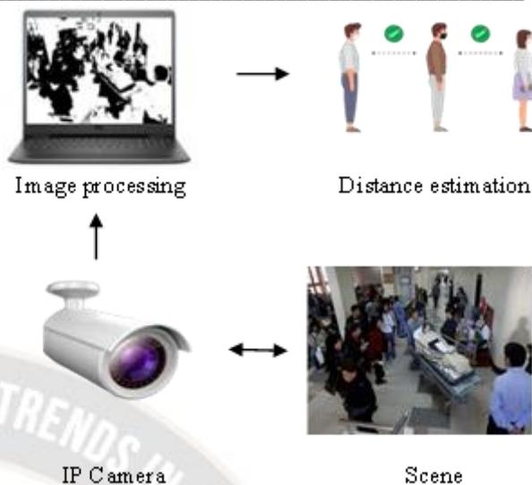
Figure 4. Distance sensing system
