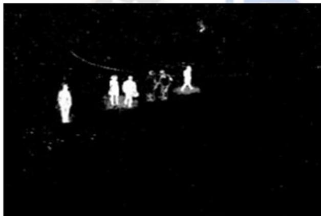
Figure 3. Image with background subtraction
