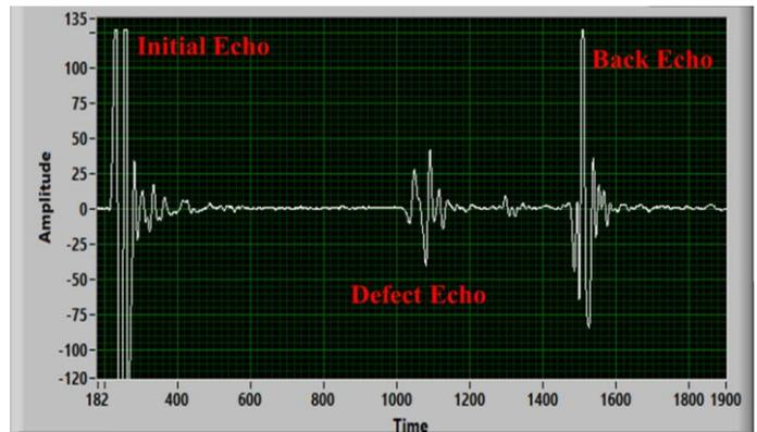
Figure 3: A-Scan signal obtained from the defect location in the welded region (normal beam technique).
