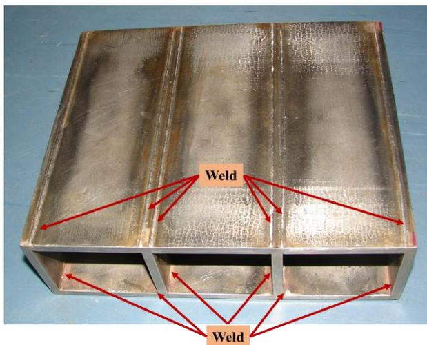
Figure 1: Photograph of the box structure
