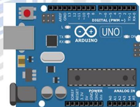
Figure 2. Pin Configuration of Arduino Uno.
