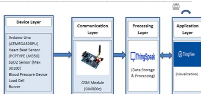
Figure 1. Architecture of Smart Maternal Monitoring Device..
