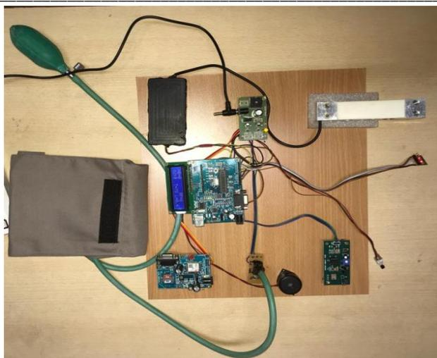
Figure 4. Smart Maternal Monitor – The Proposed Device.
