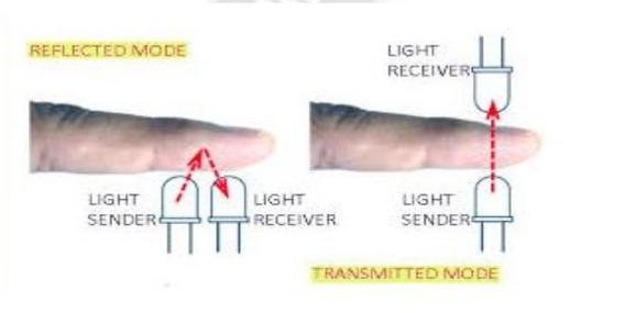
Figure 3. Operation Modes of Infrared Photodiodes.
