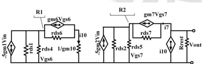
Figure 5. Small Signal model of first stage
