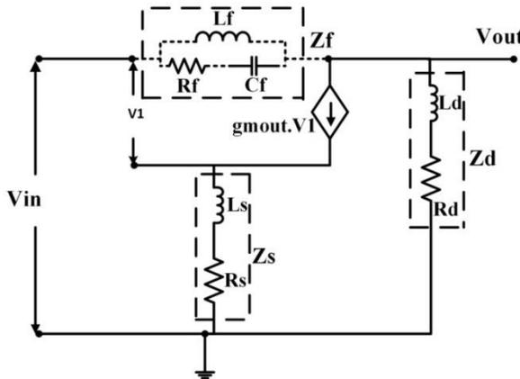
Figure.6.Small signal model of second stage
