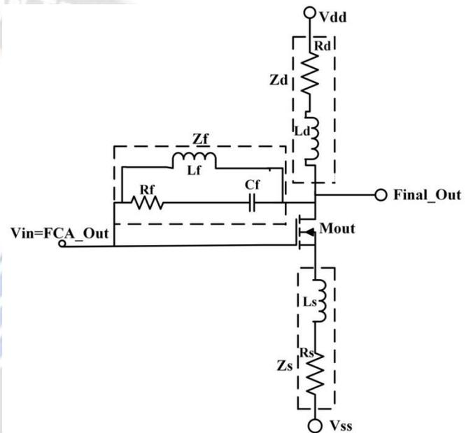
Figure 3. Schematic equivalent diagram of second stage
