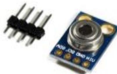
Figure 3. MLX90614 IR Temperature Sensor
