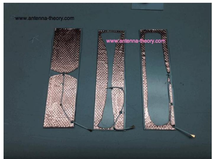
Figure 3: Design of wearable antenna
