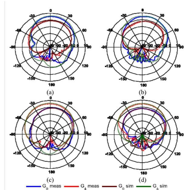
Fig 5: Fig. 8. Off-body mode radiation pattern (gain scale) at 2.45 GHz. Left: freespace; right: on-phantom (a) and (b) yz (c) and (d) xz
