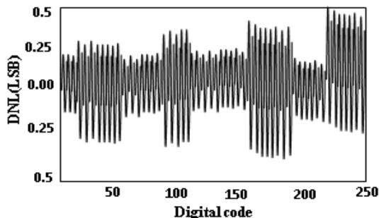
Figure 2(a). DNL Versus output Code
