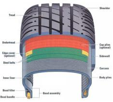
Figure 2. Constructional features of tire
