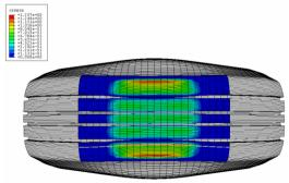
Figure 5. 3D Footprint result of Tire
