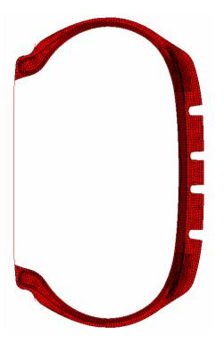
Figure 3. Axisymmetric FE-model after inflation
