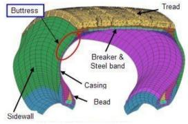
Figure 4. 3D Finite Element Model
