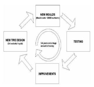
Figure 1. Traditional tire R&D process
