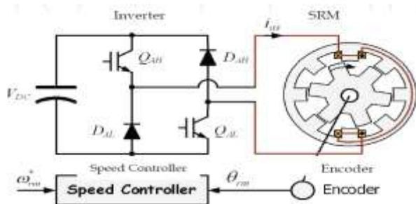
Fig.1 SRM with one phase asymmetric converter
