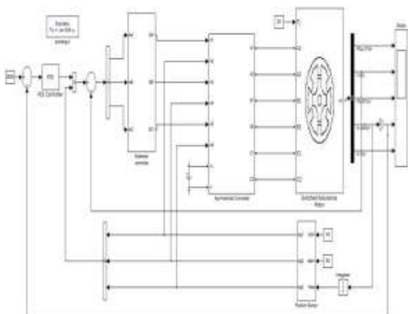
Fig. 6 Simulink model of SRM drive with PID control
