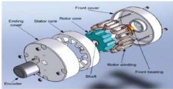
Fig.3. Construction diagram of SRM
