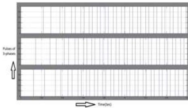
Fig. 17 Output of Position Sensor
