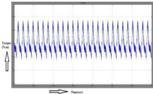
Fig. 24 Toque waveform with PID controller
