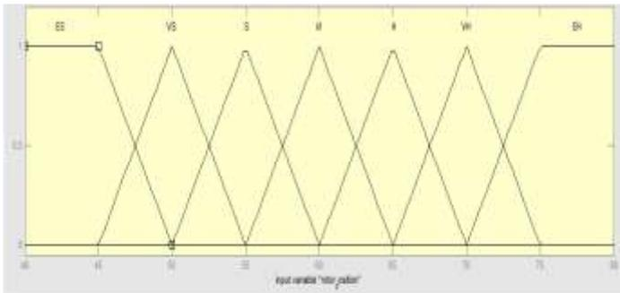
Fig. 11 Membership functions of Rotor Position
