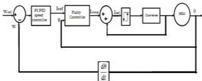
Fig. 4 Block diagram of SRM with Controller
