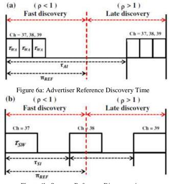
Figure 6b: Scanner Reference Discovery time
