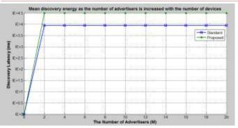
Figure 11b: Mean discovery energy as the number of advertisers is increased with the number of devices (N =  $5,\tau SI = 2560, \tau SW = 640, \tau AI = 1280$ )
