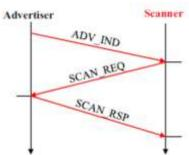
Figure 2: BLE Discovery Process
