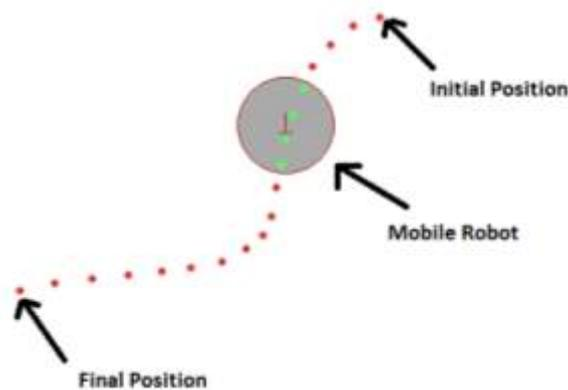
Figure. 3. Robot moves through the path of RFID tags.
