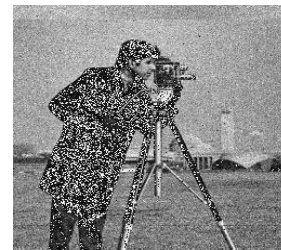
Fig 6:output image for 16PSK when snr=0
