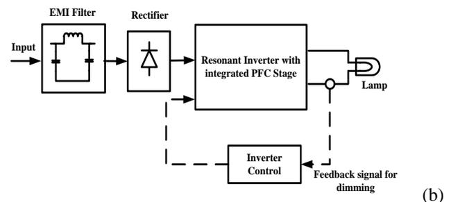
Fig.1. Typical electronic ballast systems. (a) Two-stages ballast circuit. (b) Single-stage electronic ballast.
