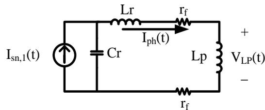
Fig. 4. Equivalent circuit before lamp ignition
