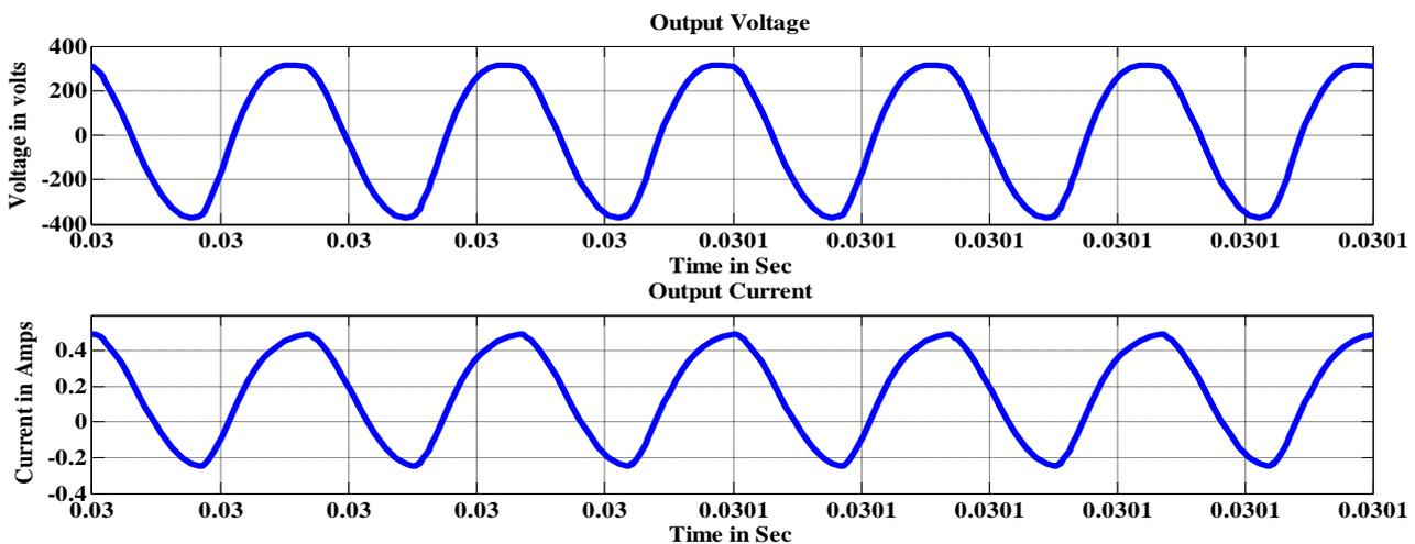
Fig.6. Lamp voltage and lamp current
