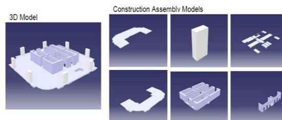
Fig. 1. Decomposition of 3D building model
