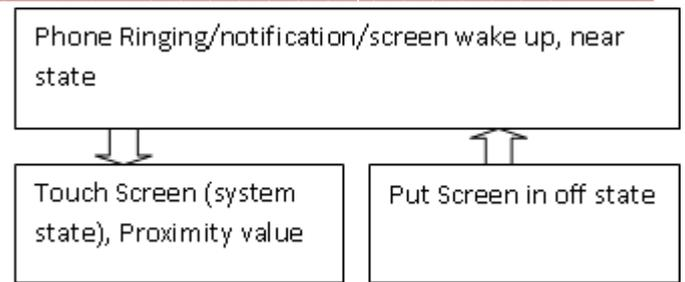
Figure 3. Close environment Control flow
