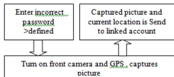
Figure 4. Un-Authentication Alert Control flow
