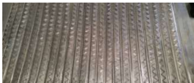
Figure 2.2 Rib-Grooved Roughened geometry absorber plate
