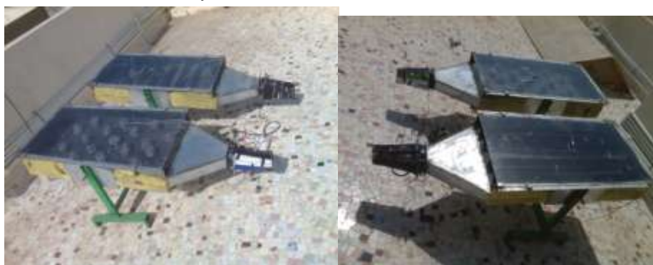
Figure 3.1. Experimental Setup Metallic Wiry Sponge Vs Baffle Type Solar AIR Heater
