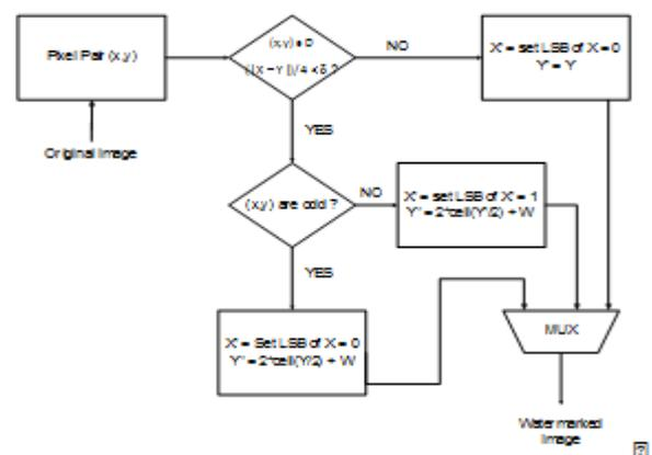
Figure 1:- Data flow of watermark embedding
