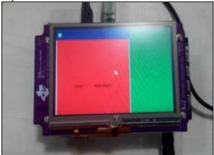
Figure 6 QML test application on am335x starter kit
