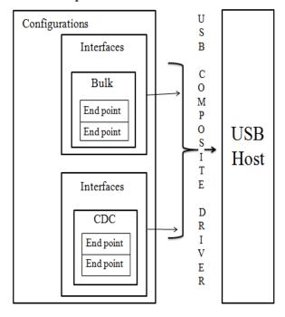
Figure 1. USB Composite Device and Host Architecture
