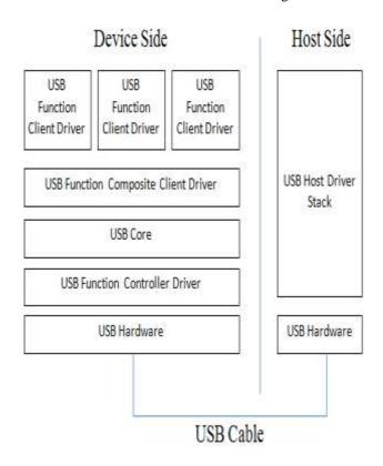
Figure 2. USB Host and Device Stack
