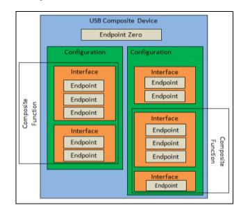
Figure 1. Composite USB Device
