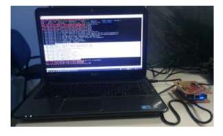
Figure 3. BeagleBone Connected to Linux PC
