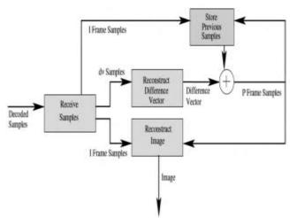
Figure 4. Block diagram for CS video decoder.[3]
