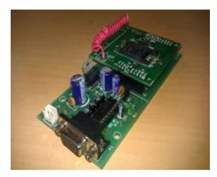
Figure.4 GSM Module
