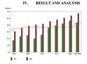
Fig.1 Emissions from bad board (failing FCC class A limits)
