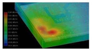
Fig5. Reduced E field radiation from good board
