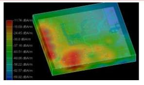
Fig.3 H field radiation from bad board at 1GHz
