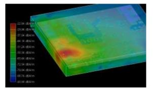
Fig.6Reduced H field radiation from good board
