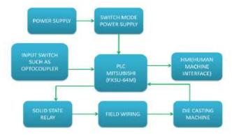
Fig.1: Block Diagram of the proposed PLC.
