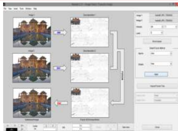
Fig4: -true color image with 750*500 pixel based process with diabetes filter, min-max fusion method and 2 level of decomposition.
