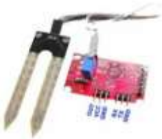
Fig. 3 Soil Moisture Sensor
