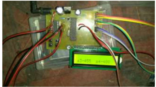
Figure 5 Working Model of Automatic Irrigation System
