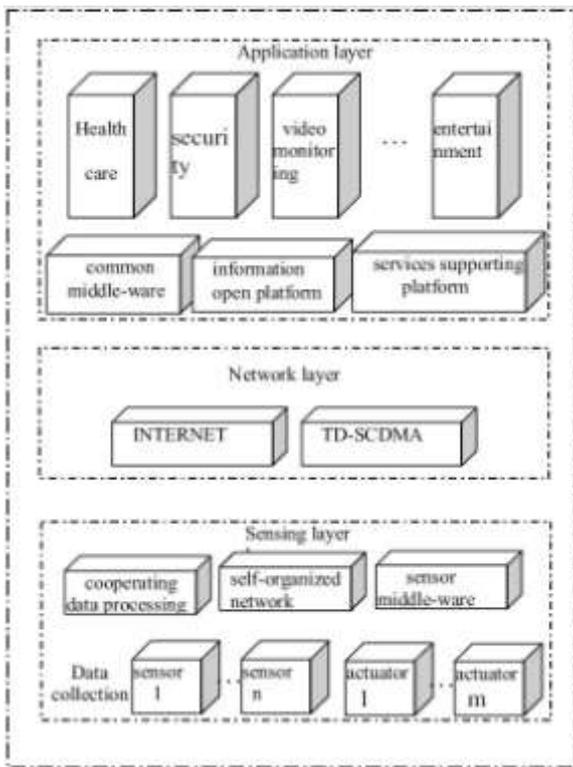
Fig. 2. Layer based Architecture of IoT [12]
