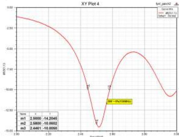
Figure 5: Return loss(dB) of an antenna without meta-surface
