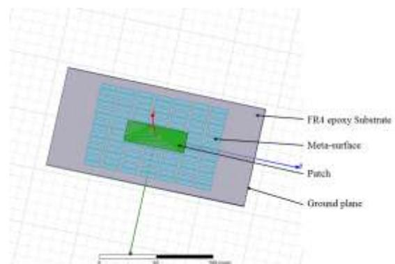
Figure 4: Rectangular patch antenna with meta-surface
