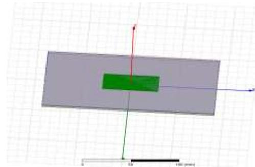
Figure 3: Rectangular patch antenna without meta-surface
