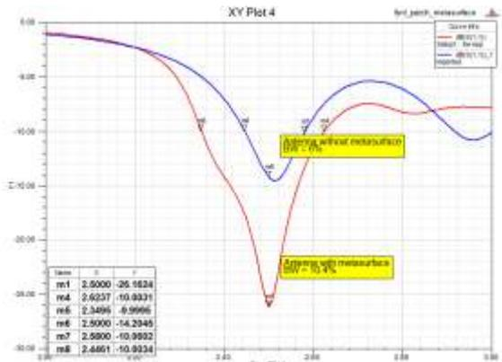
Figure 9: Return loss(dB) of a meta-surface antenna
