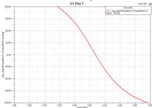
Figure 2: The reflection phase diagram of meta-surface unit cell
